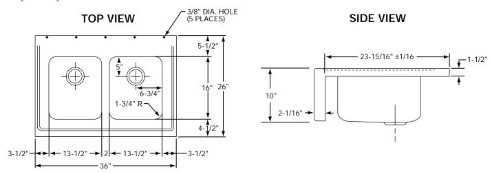
ALL DIMENSIONS IN INCHES, TO CONVERT TO MILLIMETERS MULTIPLY BY 25.4.
